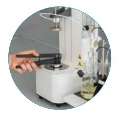
Why semi-automatic? The user places the sample in the oven with the flanging tongs and starts the method on the titrator or (optionally) on the TitriSoft software. Apart from entering the sample designation and, if necessary, the initial weight, this is all that needs to be done in the next few minutes-
