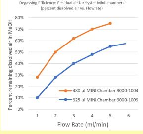
Plot shows remaining dissolved air in methanol using a selection of Systec Mini-Chambers\*. The range of chambers and specifications offered provide ample solutions for system designs.
