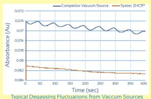
Fluctuations in detector baseline of a single-speed pump compared to the patented technology of the Systec ZHCR® pump.\* UV detector baseline fluctuations are minimal when compared to traditional stop and start vacuum sources.
