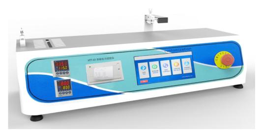
HTT-01 Hot Tack Tester is applicable in hot tack and heat seal performance tests for plastic films, laminated films and other packaging materials. It is applicable in peel test, tensile at break test, and other tests for adhesives, adhesive tapes, laminated films, plastic films, paper and other flexible materials.
