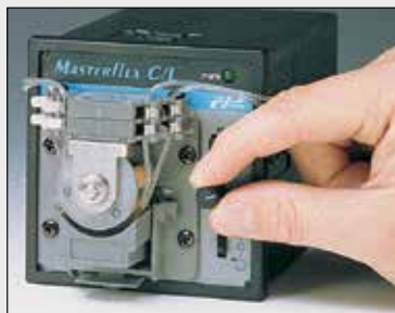
2. Snap occlusion bed shut.
