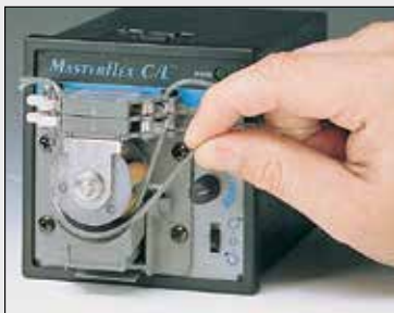
1. Lower occlusion bed. Wrap tubing around rollers and secure tubing retainers.
