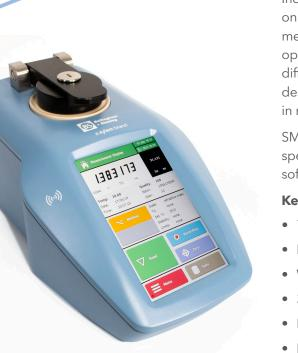
A range of touchscreen enabled digital refractometers with Peltier temperature control for high precision operation in demanding food, beverage & other industrial applications.
