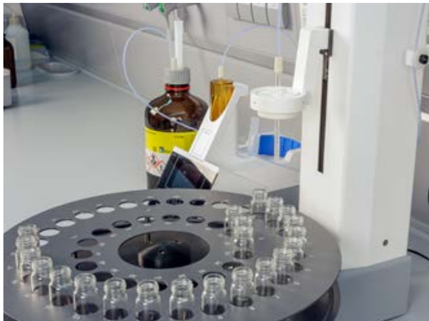
TZ4050 sample tray for VZ7088 laboratory bottles
