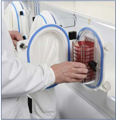
Insert 10 Plates through the glove port
