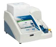
The OsmoTECH XT was designed in collaboration with customers to provide an easy-to-use instrument that can detect osmolality in a wide range of samples. OsmoTECH XT uses Intelligent freezing technology to monitor, control and measure samples with high concentration/viscosity. The instrument is ideally suited for laboratories that need to measure a wide variety of sample types across bioprocessing and cell and gene therapy workflows.
